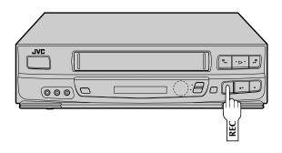
This easy method lets you record for from 30 minutes to 6 hours (selectable in 30-min. increments), and shuts the VCR off after recording is finished.
