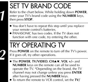
• To return the remote to VCR control, set the TV/ CABLE/VCR switch to VCR.
