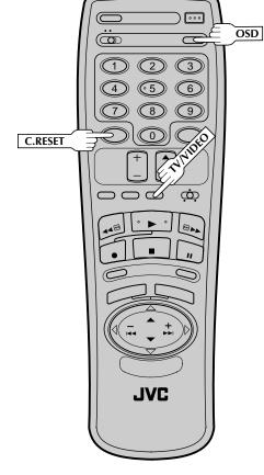
**RESET COUNTER TO ZERO** Before recording starts, press **C.RESET.** The counter resets to zero and displays the exact elapsed time as the tape runs.
